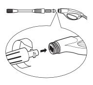
**Step 2** Slide the wand extension into the gun. Turn the wand collar clockwise onto the gun threads until tight.
